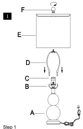
Insert the Harp (D) into the Saddle (B). Put the shade(E) on the Harp(D), then tighten the Finial (F)into the Harp (D)
