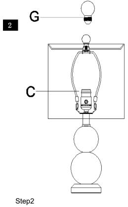
Insert the bulb(G) into the socket(C).
