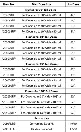
2060 Commercial Grade Pocket Door Frame for 1<sup>1</sup>/<sub>8</sub>" to 2<sup>1</sup>/<sub>4</sub>" Thick Doors to 400 lbs. (2" x 6" Stud Wall)
