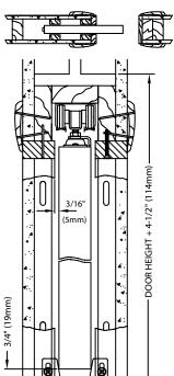
For 2 x 4 Construction. Removable aluminum track with convex rails for smooth quiet operation, rust resistant steel reinforced wood split studs, jump proof three wheel (1" dia.) hangers, self adjusting floor anchors, 2'6" and 3'0" headers marked to cut to smaller door sizes. Brass-tone steel parts. All frames for doors up to 1%" can be converted for 134" doors with 1575PPK3 adaptor kit. All oversized frames include 1575PPK3 adaptor kit.
