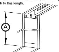
**2 OPEN** door fully (door will protrude into opening) and cut split jambs to "B" Fasten to front edge of frame. Maintain minimum 3/16" (4.7mm) clearance on both sides of door. Raise or lower hangers to plumb door with split jambs.
