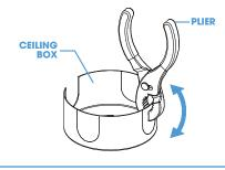
Use a plier to remove two pre-removable metal sheets on the opposite sides of the ceiling box
