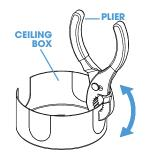
Remove the two pre-removable metal sheets on opposite sides of the ceiling box using pliers
