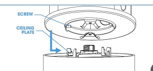
Fix the fixture onto the ceiling plate in the direction indicated by the arrow and tighten the screws on the fixture.
