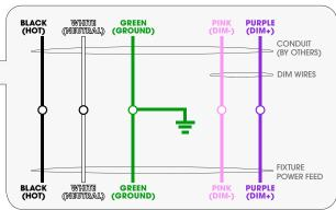
WIRING: Connect the black/while/green wires to L/N ground respectively, and connect the purple/pink wires to DIM+/DIM- respectively.
