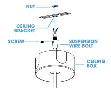
Thread the ceilng box through the suspension wire, fix the suspension wire bolt onto the wire using a screw, and secure the ceiling bracket to the suspension wire bolt with a nut
