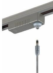
The Standard Track Adapter MA-TA-H (sold separately) enables the use of Quick Adapt Pendants in Standard, Line Voltage H-Track Systems. Includes a 50W electronic transformer. Dimmable with an electronic or standard incandescent dimmer.
