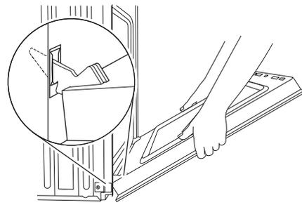
Make sure the door hinge notch is engaged on the bottom of the oven cavity slot.
