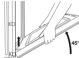
Using two hands, grasp the edges of the oven door. Close the oven door slightly past the stop position to take the weight off of the door hinges and then pull the oven door up.
