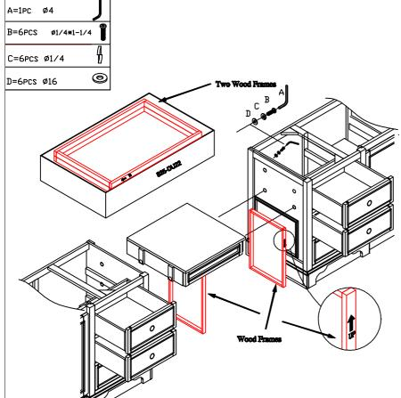
Step 3a: Locate the two rectangular wood frames included inside the carton. The frames are used to support the makeup drawer during assembly and make the installation process easier.
