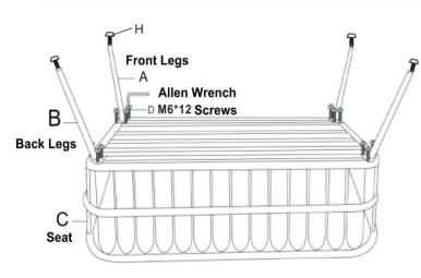
STEP 1: Attach (2) Front Legs (Part A) and (2) Back Legs(Part B) to the underside of the Seat (Part C) using (12) M6\*12Screws (Part D). Tighten using Allen Wrench (Part G).
