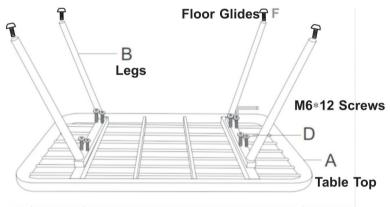
STEP 1: Attach (2) Legs (Part B) to the underside of Table Top (Part A) using (8) M6\*12 Screws (Part D). Tighten using Allen Wrench (Part E). Insert Adjustable Glides (Part F) and turn to desired height to level the table.
