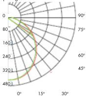
Tested at 25°C Ambient in accordance to IESNA LM-79-2008
