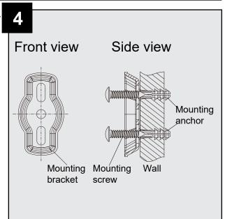
5. Place base over mounting bracket and tighten the set screw.
