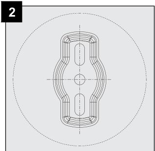
3. Drill 1/4 in. holes in drywall through the mounting screw holes. If attaching onto a wood wall, fasten mounting bracket directly to the wall with screws (included) without pre-drilling the holes.
