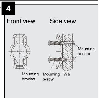
5. Place base over mounting bracket and tighten the set screw.
