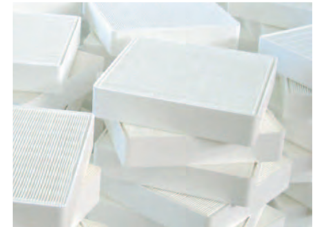
Filters awaiting final sealing process
