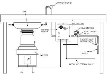
**NOTE:** The CC-202 control center should be mounted 1-1/2" (38.1 mm) back from the front surface of the table.
