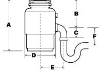
Centerline of disposer discharge to centerline at waste pipe entering wall. F٠ (Dimension "F" must be greater than 1/4" to prevent standing water in disposer.)
