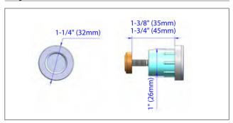
• 1-1/4"(32mm) diameter spring-loaded dust proof strike provides ample space to receive 1/2"(13mm) bolt and allows easy locking by end user
