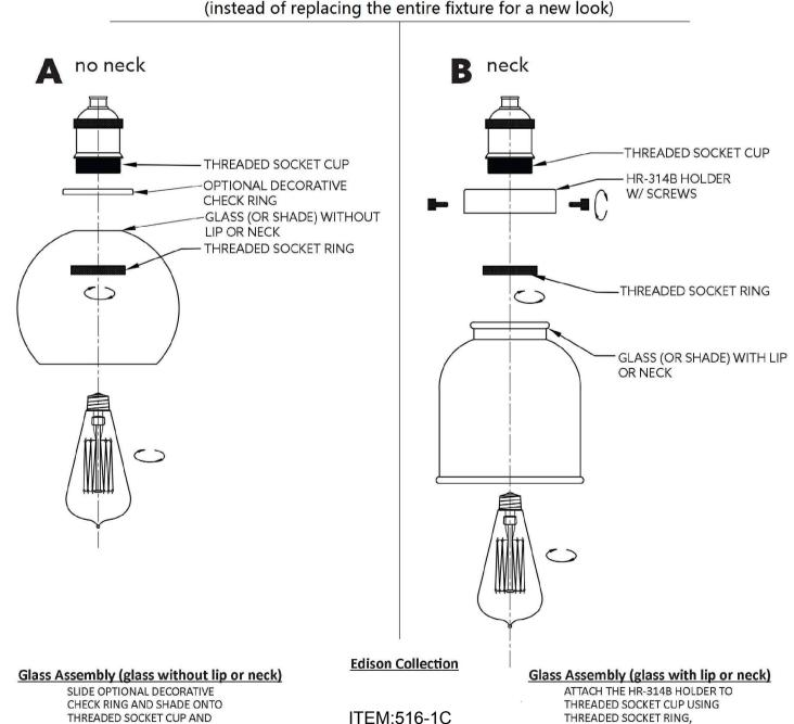
THREADED SOCKET CUP AND SECURE USING THREADED SOCKET RING DO NOT OVER TIGHTEN THREADED SOCKET RING TO
