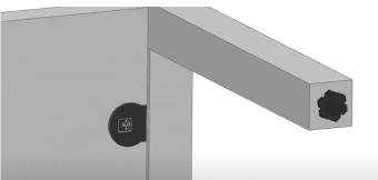
Predrill and install drywall anchors – we suggest an 8mm - 1/8 inch bit (not necessary if mounting into studs) – screw the vanity to the wall.
