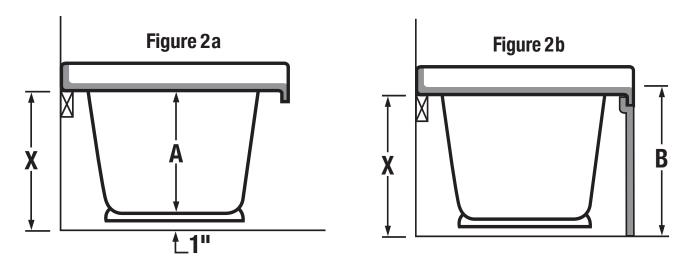
For installations that are any combination of decks, walls, and pony walls, use the same methods to determine critical heights. Remember that all supports must be at the same height and must establish a plane that is level front to back and side to side.
