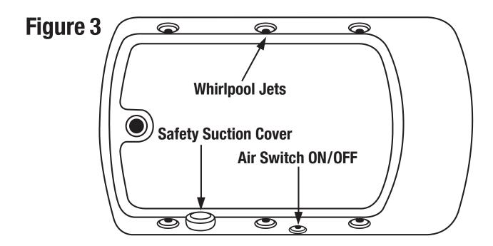
**WHIRLPOOL JETS** - These have fully adjustable direction. By rotating the jet escutcheon, this will open/close the flow of water to that jet, point the eyeball in the desired direction.
