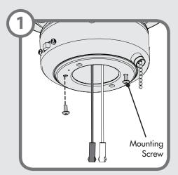
Partially install the two mounting screws into the bottom of the lower switch housing.
