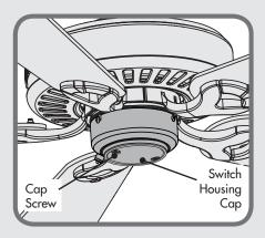
If your fan's switch housing cap resembles this one, remove the cap screws with a Phillips head screwdriver. Then follow the **TYPE-A ASSEMBLY INSTRUCTIONS** on pages 4-5.
