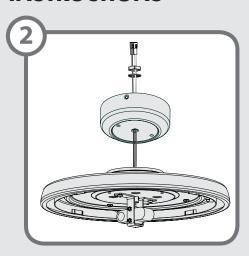
Feed the wires through the center hole in the switch housing, the washer, and the nut. Install the switch housing by twisting clockwise onto the threaded rod. Install the washer and nut onto threaded rod and tighten securely.
