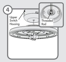
Lift the light kit up, tucking the wires into the hole in the switch housing. Install the center stem of the light kit into the lower switch housing by turning the threaded rod clockwise into the threaded hole.
