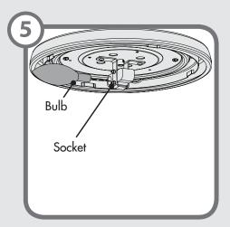
**Installing the bulbs** - Install a bulb into each of the sockets. When necessary, replace with bulbs of same type and wattage.
