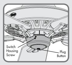
If your fan's switch housing cap resembles this one, remove the whole switch housing by removing the switch housing screws with a Phillips head screwdriver. Remove the plug button. Then follow the TYPE-B ASSEMBLY INSTRUCTIONS on pages 6-7.
