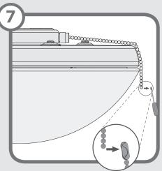
Installing the pull chain pendant -Attach the pull chain pendant to the end of the short chains coming from the switch housing and the light kit.
