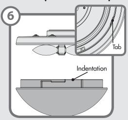
Installing the globe- Position the indentations in the outer rim of the globe so that they line up with the tabs on the inside surface of the light fixture rim.
