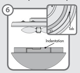
Installing the globe- Position the indentations in the outer rim of the globe so that they line up with the tabs on the inside surface of the light fixture rim. Carefully lift the globe up inside the light fixture as far as it will go. Rotate the globe in a clockwise direction until it is held tightly in place by the four tabs.
