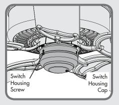
If your fan's switch housing cap resembles this one, remove the whole switch housing by removing the switch housing screws with a Phillips head screwdriver. Remove the two cap screws from the inside of the switch housing. Reinstall the switch housing. Tighten the switch housing screws. Then follow the TYPE-A ASSEMBLY INSTRUCTIONS on pages 4-5.
