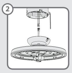
Feed the wires through the center hole in the switch housing. Then using the single pin connectors, connect the black or blue wire from the fan to the black wire from the light kit. Connect the white wire from the fan to the white wire from the light kit.
