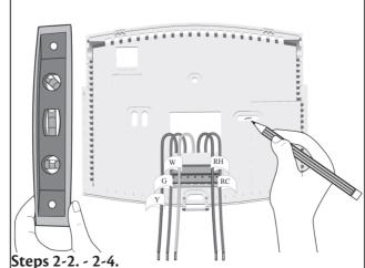
2-5. Remove the wall plate and drill two 3/16" holes where marked.
