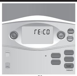
7. Auto recovery – allows heating and cooling systems to gradually recover from an energy-saving setpoint temperature to a comfort setpoint temperature. Auto recovery calculates the time needed to adjust the temperature to the next program setting. When the thermostat is in Auto Recovery mode, the display will flash alternating messages of RECO and the time. Auto Recovery can be disabled by sliding the recovery switch on the back of the circuit board to the disable position.
