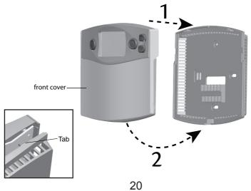
4. Place the top of the thermostat over the two tabs on the wall plate. Press the thermostat onto the wall plate and press to snap the bottom tab into place.
