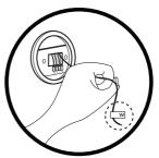
NOTICE! Do not disconnect the wires from the existing thermostat before reading these instructions. The wires must be labeled prior to removal to ensure proper reconnection.
