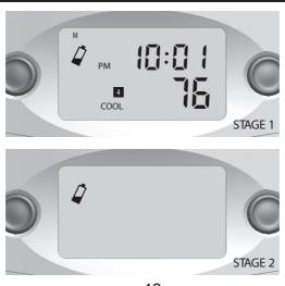
Low battery warning – indicates two stages of battery power shortage.
