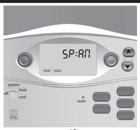
5. Span setting mode – allows you to adjust the system ON/OFF cycle rate. The default setting is 2 (the system cycles ON or OFF when the temperature is within 1<sup>o</sup> F (0.5<sup>o</sup> C) above and below the set temperature.) The span setting can be adjusted if your system is cycling too fast or too slowly.
