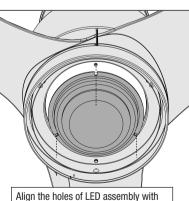
Align the noies of LED assembly with the holes of the upper switch housing. Make sure all the wires from the fan and the light kit are snug insinde the center of the light kit, not pinched in between the upper switch housing and the light kit or hanging out or the sides.
