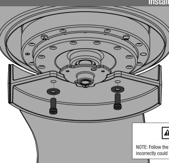
Put the blade washers found in the hardware bag onto the blade screws found in the hardware bag. Then install the blade screws to secure each blade to the fan.
