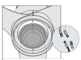
Connect the singlepin connectors to the connectors from the fan.
