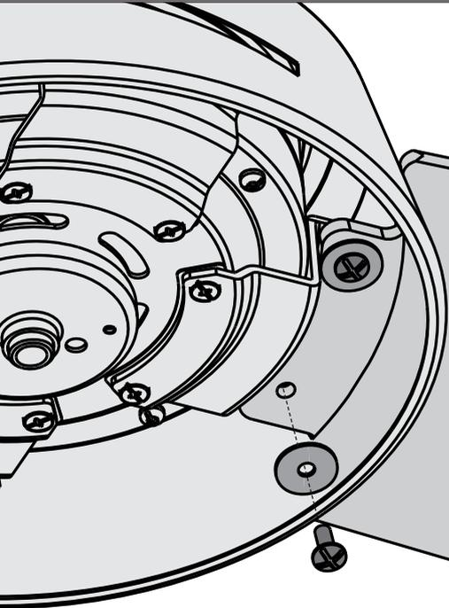
Attach each blade to a blade iron using three blade washers, found in the ■ hardware bag, and three blade assembly screws, found in the ▲ hardware bag.
