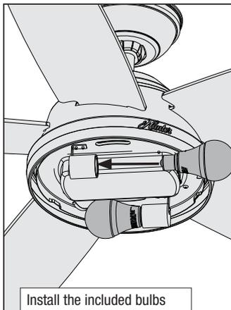
Install the included bulbs into the sockets. When necessary, replace with bulbs of same wattage.
