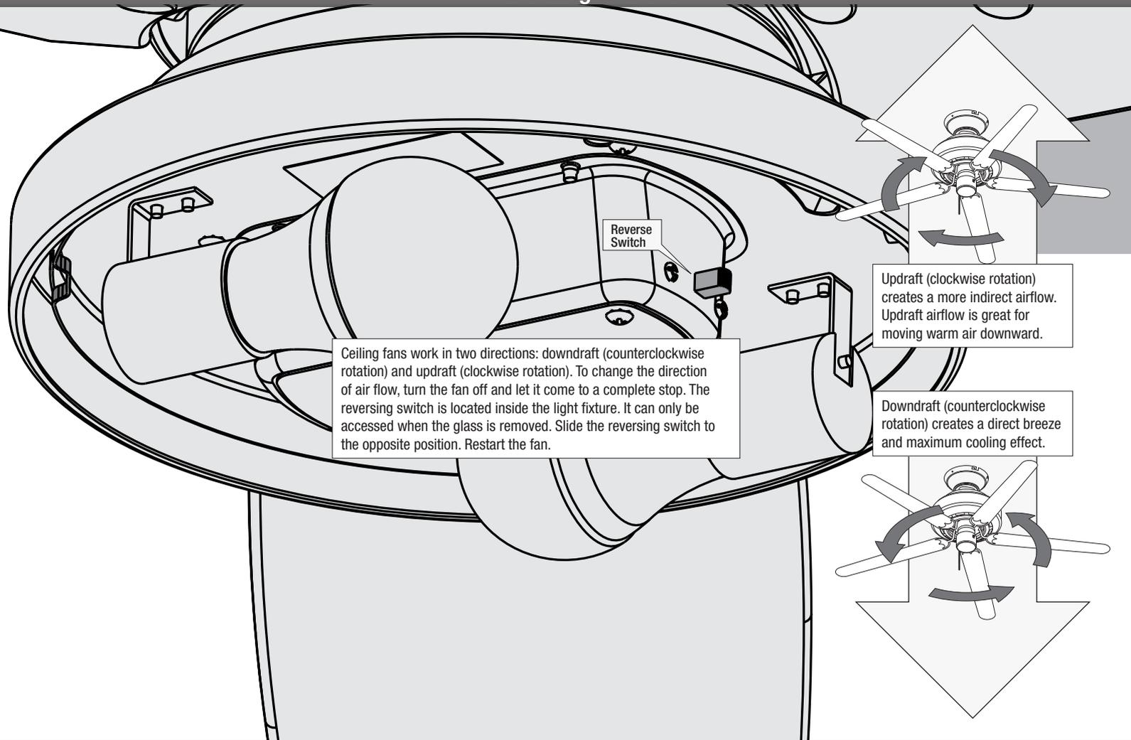
Ceiling fans work in two directions: downdraft (counterclockwise rotation) and updraft (clockwise rotation). To change the direction of air flow, turn the fan off and let it come to a complete stop. The reversing switch is located inside the light fixture. It can only be accessed when the glass is removed. Slide the reversing switch to the opposite position. Restart the fan.
