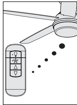
The remote transmitter is already paired to the receiver and ready to use. **Dimming mode is off by default.**
