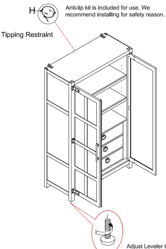
Adjust Leveler if needed to level wardrobe on uneven floor.
