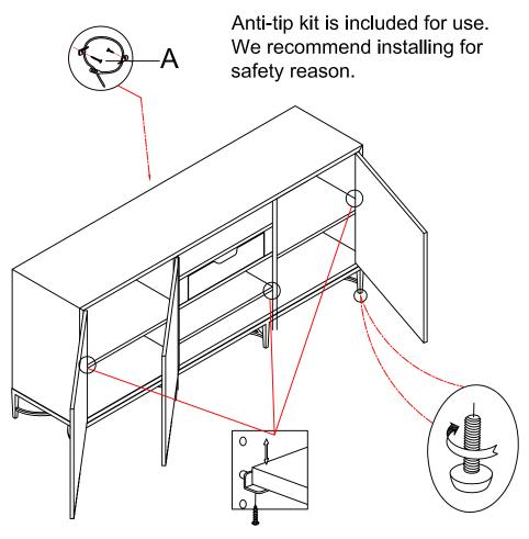
The adjustable shelves are screwed in place to avoid damage during transit. To adjust the shelf height, remove screws then place shelf pins in the desired level.
