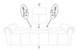
STEP 1 - Place Bracket into Sleeve and presstop of back down firmly to lock your KD back in place
