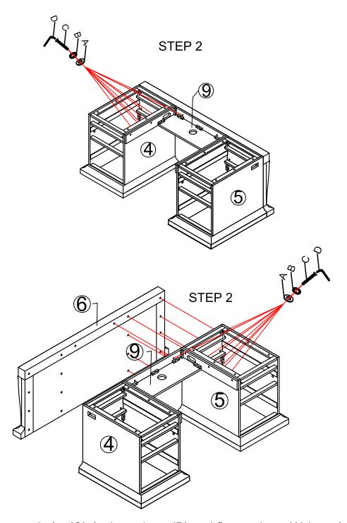
Step 2: Loosen bolts (C), lock washers (B) and flat washers (A) by using allen wrench (D), then remove back panel (6) from the desk.
