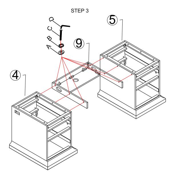
Step 3: Loosen bolts (C), lock washers (B) and flat washers (A) by using allen wrench (D) from the left and right bases (4, 5), well remove the center section (9).
