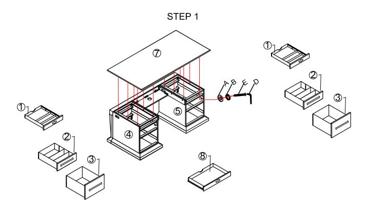
Step 1: Take out all drawers (1, 2, 3, 8), then loosen bolts (E), lock washers (B), and lock washers (A) on the wood cleats by using allen wrench (D) and remove top panel (7) from the desk.
