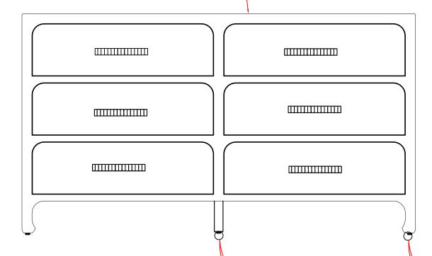
Adjust leveler if needed to level dresser on uneven floor.
