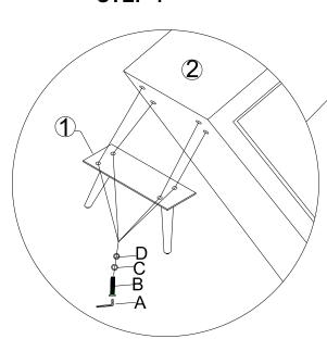
Adjust leveler if needed to level door chest on uneven floor.
