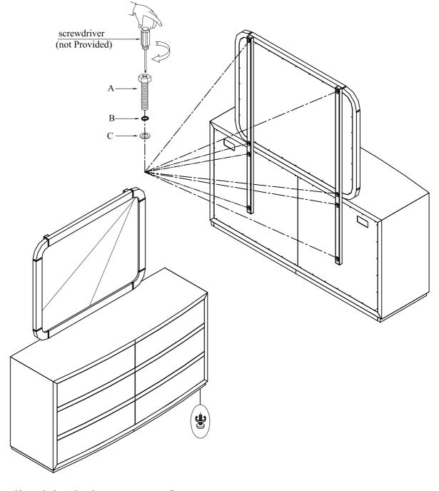
Adjust levelers if needed, to level case on uneven floor
