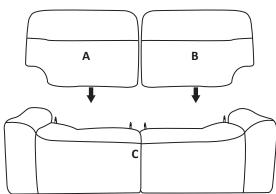
**Step3** Slide the metal inserts on the LAF Wing and RAF Wing into the metal sleeves on the side of the LAF Back and RAF Back. Slide the wings down until they are completely set on the backs metal sleeves.
