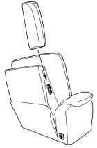
**Step4** Attach the leadwires found at the bottom of motion back to the leadwires at the rear of seat. Yellow to Yellow & Grey to Grey. Make sure to close the clip locks to assure the connections will not come loose during use.
