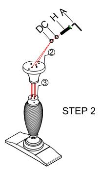
Step 2: Unscrew the assembly hardware as shown in diagram, then remove extension block (2).
