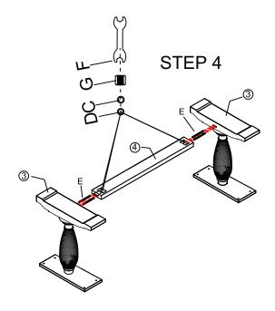
Step 4: Attach stretcher (4) between the pedestals (3).
