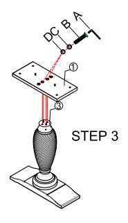
Step 3: Re-assemble the mounting bridge (1).
