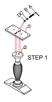
Step 1: Unscrew the assembly hardware as shown in diagram, then remove mounting bridge (1).
