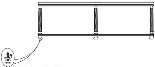
Adjust Leveler if needed to level table on uneven floor.
