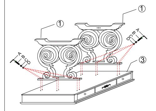
Step 1: Attach bases (1) to desk top (3) by using flat washers (D), lock washers (C) and bolts (B), turn the bolts (B) with allen wrench (A). Do not fully tighten bolts (B) at this step.
