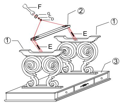
Step 2: Insert threaded rod (E) through hole on each end of stretcher (2) to the hole on each base (1), well insert flat washers (D), lock washers (C) and nuts (G) through threaded rods (E). Turn the nuts (G) with spanner (F). Do not fully tighten nuts at this step.
