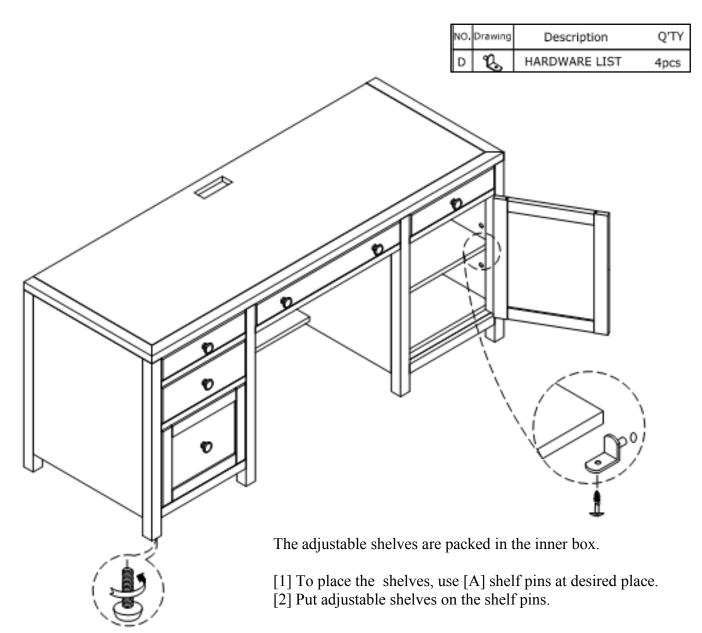
Adjust center leg & levelers if needed to level case on uneven floor.
