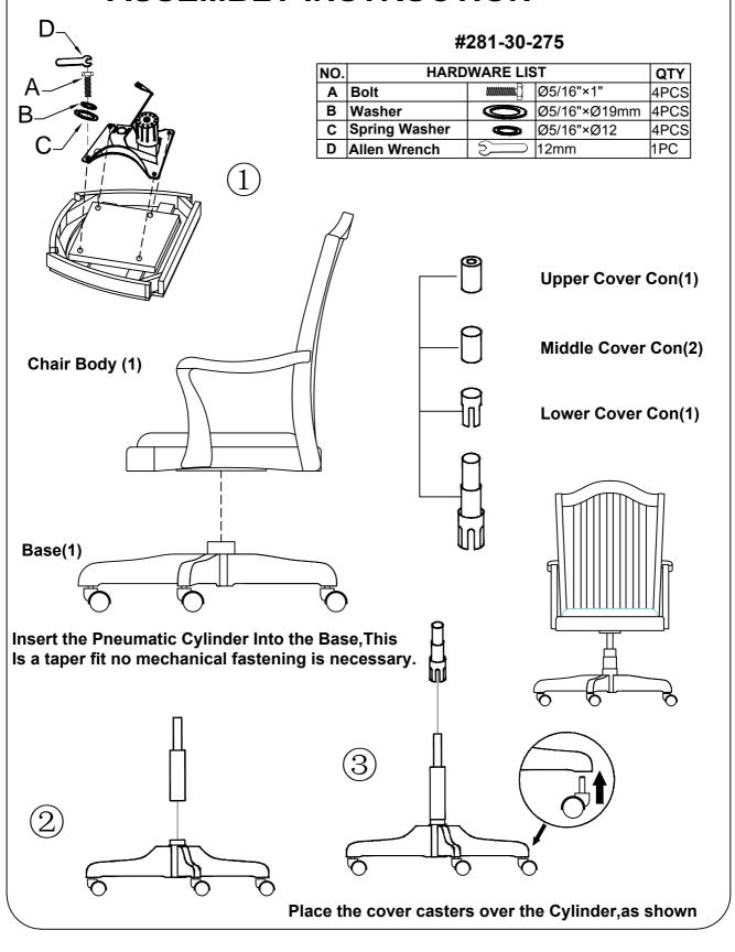
Place the chair body onto the cylinder. No mechanical fastening is necessary because this is a taper fit . Now sit in the chair. This will firmly secure the taper fit.
