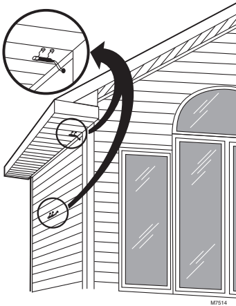
Fig. 1. Typical locations for outdoor sensor.
