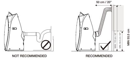
**WARNING:** Any warranties included with this product will be voided if an extra extension hose is added to the originally provided installation kit or if the installation is performed differently than the manufacturer's instructions, without proper consultation. Please contact Customer Support for help with installation if needed.
