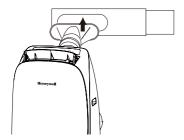
Connect the plastic hose to the hose connector on back of the unit. Slide-in the hose connector downwards until it is locked in place.
