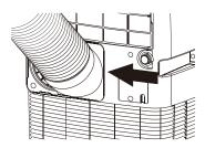
4 Connect the window bracket to the opposite end of the plastic hose. Ensure that all connections are tight and installed properly.
