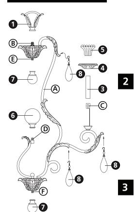
\*\*\* The construction of this fixture will be accomplished by first rotating the fixture arms into the correct position, assembling the basic fixture, installing the mounting hardware, making all necessary electrical connections, mounting the fixture to the ceiling and then hanging the crystals.
