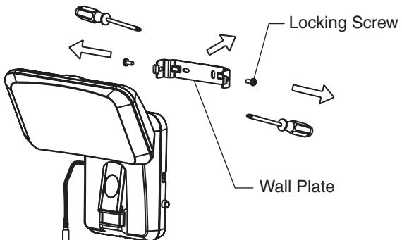
2. Use two screws and anchors to mount the wall plate to a solid surface. Make sure there is enough vertical space above the mounting plate to allow the light fixture to be mounted.
