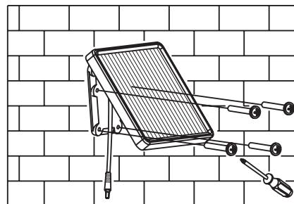
2. Adjust the angle of the solar panel by grasping the panel and gently rotating it up or down as needed. Remember, the solar panel must receive as much direct sunlight over the course of the day as possible. Keep in mind that shadows may block the sunlight from reaching the solar panel during the day.
