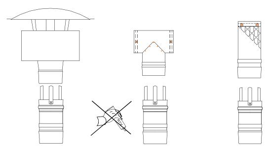
Termination attaching to EZ Seal, NO sealant required.
