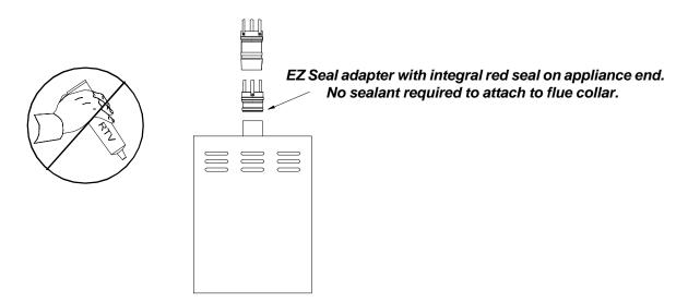
• If the integral red seal is only in the female end, you will need to use an approved high-temperature RTV silicone sealant to make the connection to the appliance. Follow the procedure recommended by the appliance manufacturer.
