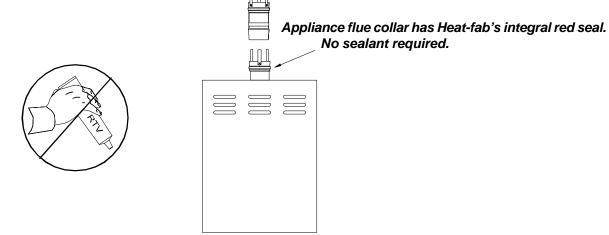
• If the flue collar has Heat-fab's female end (with the 3 tabs) but does not have the integral red seal, you will need to use an approved high-temperature RTV silicone sealant to make the joint between the flue collar and the first piece of EZ Seal. The rest of the system can be sealant-free if it is all EZ Seal.
