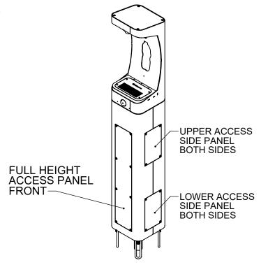
HAWS MODEL 3610/3610F IS FULLY COMPLIANT WITH THE FEDERAL 2010 AMERICANS WITH **DISABILITIES ACT (ADA) ACCESSIBILITY** REQUIREMENTS WHEN INSTALLED AS SHOWN HERE AND WHEN INSTALLED WITH PROPER **CLEARANCES AND ACCESS. IT IS THE** RESPONSIBILITY OF THE INSTALLER TO ADHERE TO LOCAL, STATE, AND FEDERAL CODES WHEN INSTALLING THIS UNIT. DISTANCE TO SURROUNDING OBJECTS, APPROACH SURFACES, ETC. SHOULD BE CONSIDERED. REFER TO SHEET 7 FOR MORE INFORMATION.
