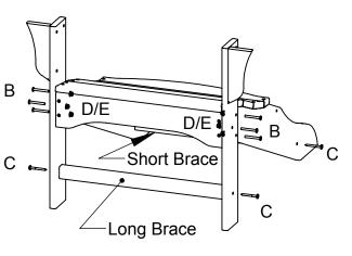
**STEP 3** Attach Back to Seat and Arms using (4) 2" screws STEP 2
