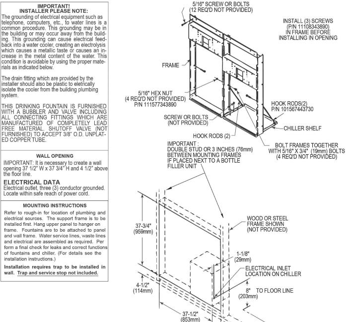
isolate the cooler from the building plumbing system. THIS DRINKING FOUNTAIN IS FURNISHED WITH A BUBBLER AND VALVE INCLUDING ALL CONNECTING FITTINGS WHICH ARE MANUFACTURED OF COMPLETELY LEAD FREE MATERIAL. SHUTOFF VALVE (NOT
