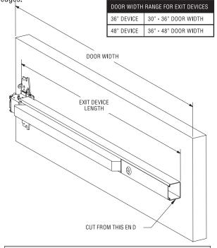
RECOMMENDED OVERALL EXIT DEVICE LENGTH = DOOR WIDTH - 4"
