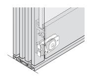
For door widths greater than 900 mm (35 7/16") it is recommended to use an additional lower guide. Refer to page 408 for detail.
