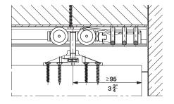
The two-way suspension bracket allows the door to be hung and to be taken off in two different ways:
