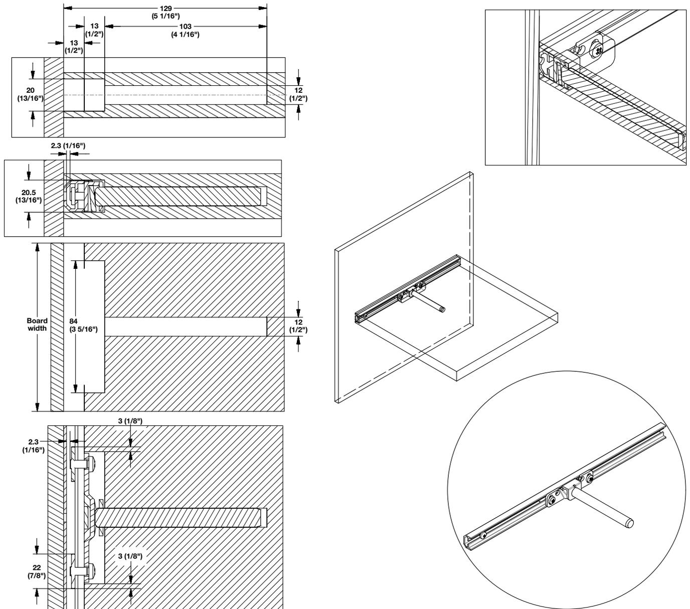
Proper routing for the shelf support and rail on rear edge of the panel will serve as an anti-tip feature when shelf is mounted. Applying a small amount of silicone adhesive will help secure the shelf support to the rail and panel.
